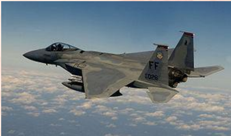
F-15 Eagle is powered by two Pratt & Whitney F100 axial-flow turbofan engines
